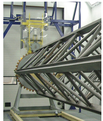
Installation prepared to paint crane parts.
