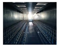
These conveyors can incorporate the *power and free* mechanism, which allows us to have total control of the feed of the workpiece.
